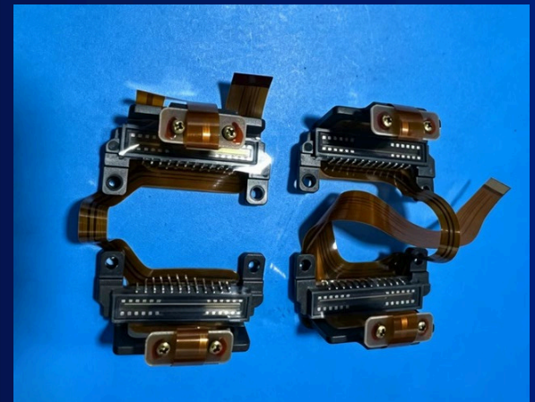
Topcon, Sokkia total station iES, FX, CX vertical, horizontal CCD.
