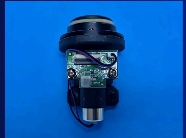
Topcon ES-602, OS-602, ES-52, ES-102, Sokkia CX-52, CX-102 universal compensators.
