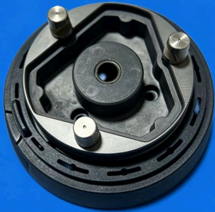
SOKKIA, Topcon total station Es, Os, cx, FX base assembly.
